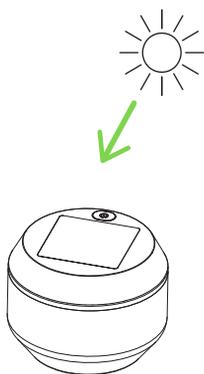
It is recommended to put the solar panel in the sun for 9 hours to charge the battery.
