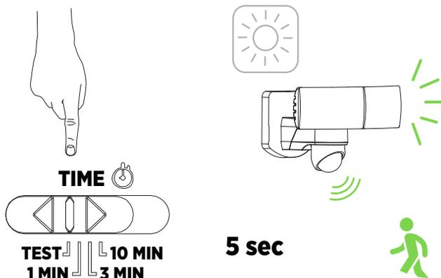
To adjust the detection zone in daylight. When the sensor detects movement the light turns on for 5 sec.
